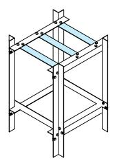
(E) ONCE ALL THE LENGTHS ARE CUT TO THE SPECIFIED DIMENSIONS, WE NEED TO DRILL ALL THE HOLE LOCATIONS TO ALLOW THESE COMPONENTS TO SCREW TOGETHER.
