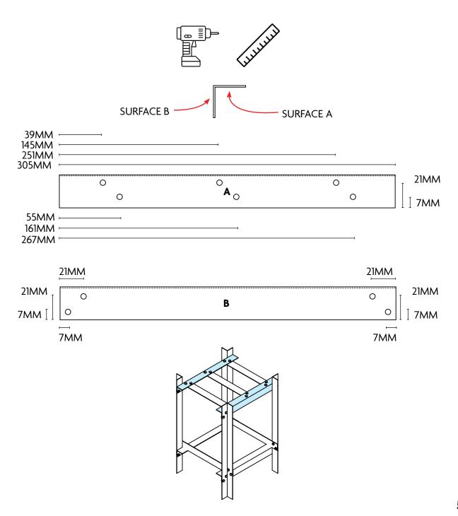
(C) ONCE ALL THE LENGTHS ARE CUT TO THE SPECIFIED DIMENSIONS, WE NEED TO DRILL ALL THE HOLE LOCATIONS TO ALLOW THESE COMPONENTS TO SCREW TOGETHER.
