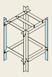
(F) ONCE ALL THE LENGTHS ARE CUT TO THE SPECIFIED DIMENSIONS, WE NEED TO DRILL ALL THE HOLE LOCATIONS TO ALLOW THESE COMPONENTS TO SCREW TOGETHER.
