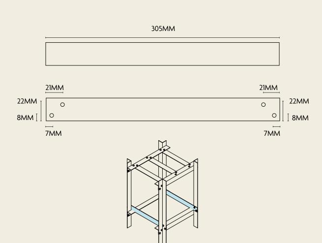
(D) ONCE ALL THE LENGTHS ARE CUT TO THE SPECIFIED DIMENSIONS, WE NEED TO DRILL ALL THE HOLE LOCATIONS TO ALLOW THESE COMPONENTS TO SCREW TOGETHER.
