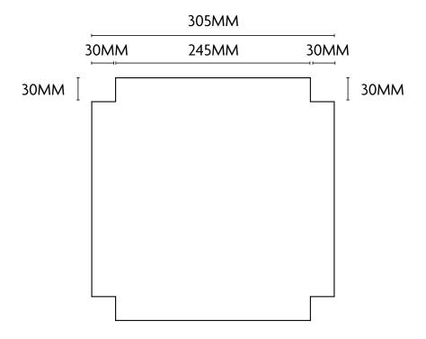
(I) FOR THE BOTTOM <u>CORK TILE</u> WE WILL NEED TO USE OUR 10MM HOLE PUNCH TO REMOVE HOLES SO THAT THE NUTS FROM THE ASSEMBLY OF THE FRAMEWORK CAN SIT WITHIN THE CORK AND ALLOW THE CORK TO SIT FLAT.
