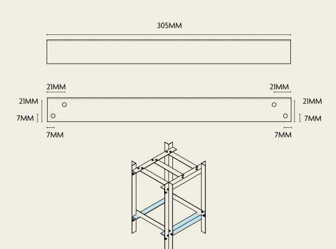
(B) ONCE ALL THE LENGTHS ARE CUT TO THE SPECIFIED DIMENSIONS, WE NEED TO DRILL ALL THE HOLE LOCATIONS TO ALLOW THESE COMPONENTS TO SCREW TOGETHER.
