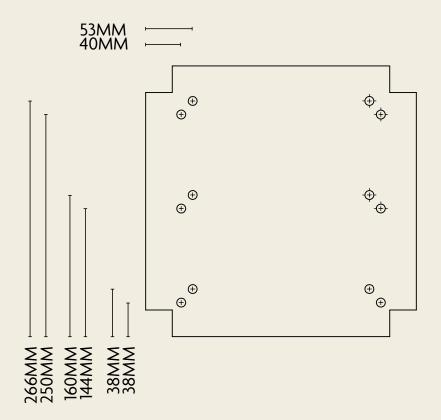
(J) LASTLY PLACE THE LAST CORK TILE AND ALIGN EACH PUNCHED HOLE TO THE NUTS OF THE FRAME AND PROCEED TO POSITION THE REMAINING FIVE CORK TILES INTO POSITION.
